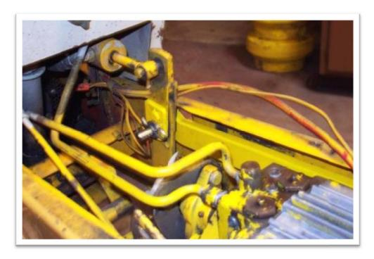
At this point, after making sure the all bolts are snug, and all wires are out of the way, you can re-attach the battery and start the tractor. CAREFULLY raise and lower the hydraulics lift and make sure that everything is clear and operates as needed. Once satisfied, tighten all the bolts that hold the rear plate on, the axle housing bolts, etc.
