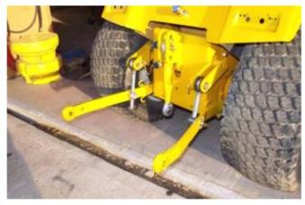
This completes the installation. Make sure that everything is tight and functions as needed. You can re-install your original hitch with some  $3/8" \times 1"$  bolts if desired. Nuts are welded to the back of the plate already.
