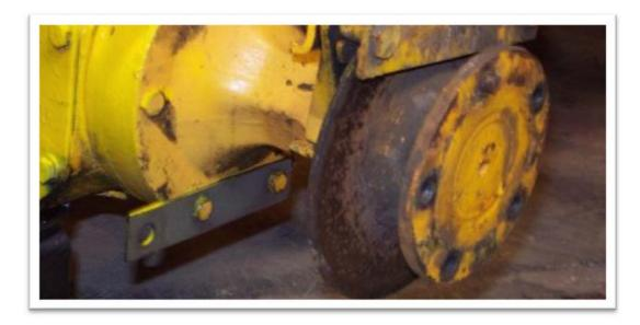
Now you can slide the plate with the rock shaft up into the frame. The plate will fit inside of the frame rails. Use the 3/8" bolts, lock washers and nuts as shown. Make the bottom bolt come thru from the inside as shown. Use the 7/16" bolts, lock washers and nuts for the larger bottom hole.
