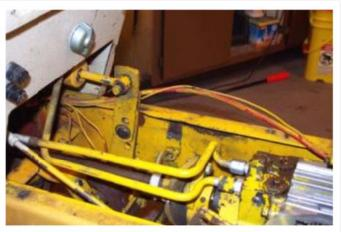
At the rear of the frame, on the right side, sometimes there is only 1 hole, and possibly no holes. These will need to be drilled with a 3/8" drill to mount the rear 3 point plate. Match the holes for location from the left side of the tractor to the right side.
