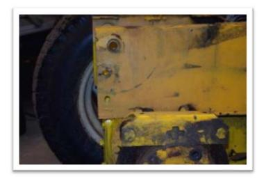
Then you will need to attach the link shaft to the rear main plate. Use a 5/8" pin and cotter pin. The pin goes thru the side of the plate, thru the rock shaft brackets.
